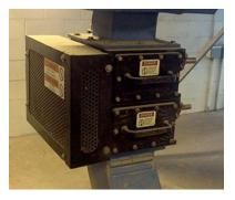
Some of the benefits included access doors on both sides of the valve, a molded cast handle to make replacing and handling the door easier, along with locating pins for lining up the holes to make starting the screws much faster. Meyer also has extended shafts on both sides that give the customer the option of left or right hand drive or even dual cylinder operation. This particular application also required safety guards which is a standard option with the Meyer offering.
